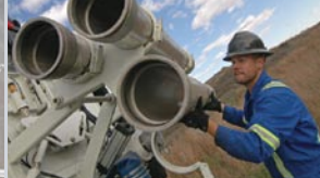
Hydraulically operated storage for 32' of vacuum tubes
