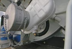
Heated decant valve with internal filter
