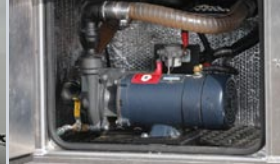
35 gpm/2000 psi water pump with variable output
