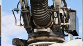
Heavy-duty reinforced boom elbow and internal material deflector
